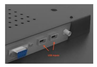
Figure 1 Position of USB ports
